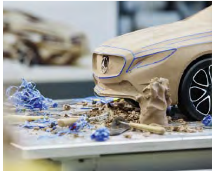
The unique sculptural quality of the new A-Class can be seen in its characteristic lines, well-defined edges, and taut surfaces. These fascinating shapes were initially handmade in clay.
